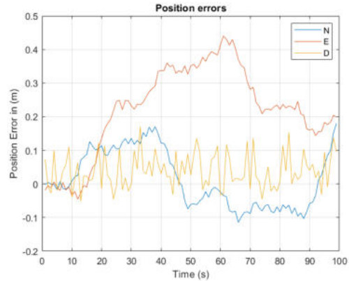
Fig. 9: Square Motion EKF Position Estimation Errors.
